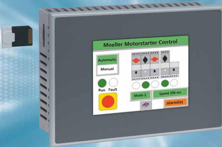
The MFD4-5-XRC-30 multi-function display is a new component in Moeller's automation range. The device from the easyHMI device series features a full graphics 5.7 inch colour STN display with 256 colours, resistive touch technology as well as a host of communication options.
